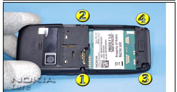
8. Tighten the screws with a torque of 19Ncm in the order shown.
