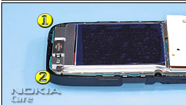
7. Insert new screws and tighten them with a torque of 17Ncm in the order shown.
